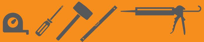
Tape measure, Philips headed screwdriver, soft / rubber headed hammer, a straight edge tool and AXIOME® compatible sealant plus a sealant gun
