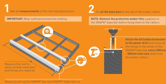
length, **30mm-40mm longer than the rafter** so they overhang into the correct position for the gutter end of the roof.
